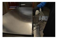
Spray a clean, sanitizer-soaked towel with Heavy Duty De-greaser solution then wipe down the out-feed rack. Rinse the out-feed rack with a separate, clean sanitizer-soaked towel.
