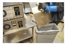
Spray a clean, sanitizer-soaked towel with Heavy Duty De-greaser solution then wipe down the in-feed rack. Rinse the in-feed rack with a separate, clean sanitizer soaked towel.
