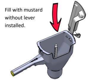
With a clean and empty dispenser add mustard BEFORE installing lever. If dispenser has run out of sauce during use it can be refilled without removing lever.
