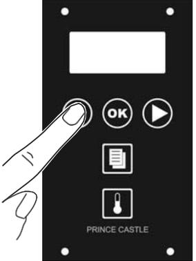
The diagram shows a hand with the index finger pressing and holding the left scroll button (a square button with a left-pointing arrow) on the toaster's control panel. The control panel includes a digital display at the top, an OK button, a right scroll button, a menu button (square with a list icon), and a temperature button (square with a thermometer icon). The brand name 'PRINCE CASTLE' is printed at the bottom of the panel.
