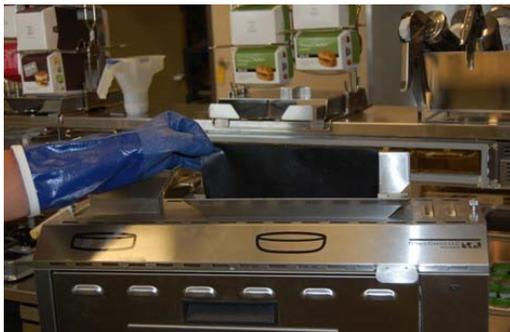
**3** **Fold and crease release sheet.** Fold release sheet in half and create a crease in the center of the sheet.
