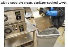
Spray a clean, sanitizer-soaked towel with Heavy Duty De-greaser solution then wipe down the in-feed rack. Rinse the in-feed rack with a separate, clean sanitizer soaked towel.
