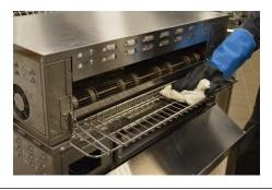
Spray a clean, sanitizer-soaked towel with Heavy Duty De-greaser solution then wipe down the exterior of unit. Rinse the exterior of unit with a separate, clean sanitizer-soaked towel.
