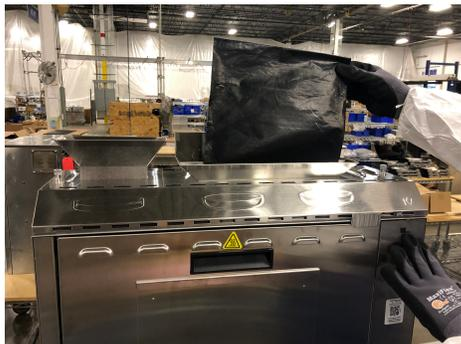
**3** **Fold and crease release sheet.** Fold release sheet in half and create a crease in the center of the sheet.
