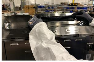
NOTE: When installing release sheet, you may flip inside-out and use the other side if needed.
