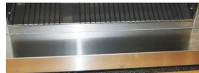
Improper Installation of Wire Bun Chute
