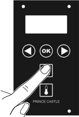
The diagram shows a hand with the index finger pressing the menu button (a square button with a list icon) on the toaster's control panel. The panel features the same layout as in the first diagram: a digital display, OK button, right scroll button, menu button, and power button, with 'PRINCE CASTLE' printed at the bottom.
