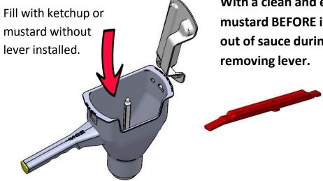
With a clean and empty dispenser add ketchup or mustard BEFORE installing lever. If dispenser has run out of sauce during use it can be refilled without removing lever.
