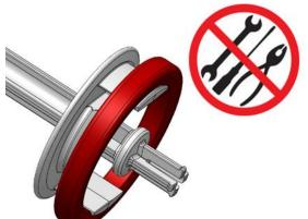
Install and replace piston ring and spring by hand, do not use tools or sharp objects. Ketchup piston ring shown.
